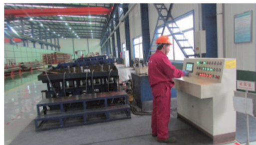
Pressure test bench
